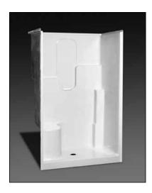
**Specification** – Oasis one-piece FRP gelcoat shower compartment SH-4836 RS or LS, having a single contoured seat and offered in a standard 4-inch or 6-inch (ABF) dam configuration. ActivLife package includes factory applied, 3-wall, full-wrap reinforcement, exceeding (HUD/FHA) 'Fair Housing' requirements.
