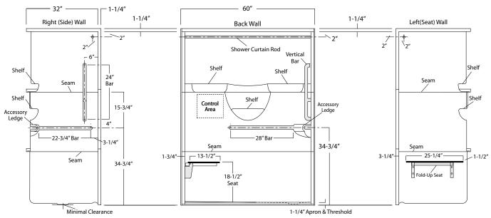
Photographic images may include optional components and appear different than actual product. Dimensions shown are maximum. Due to the nature of the materials involved, actual unit dimensions can vary (tolerances: +/-1/8 inch)
