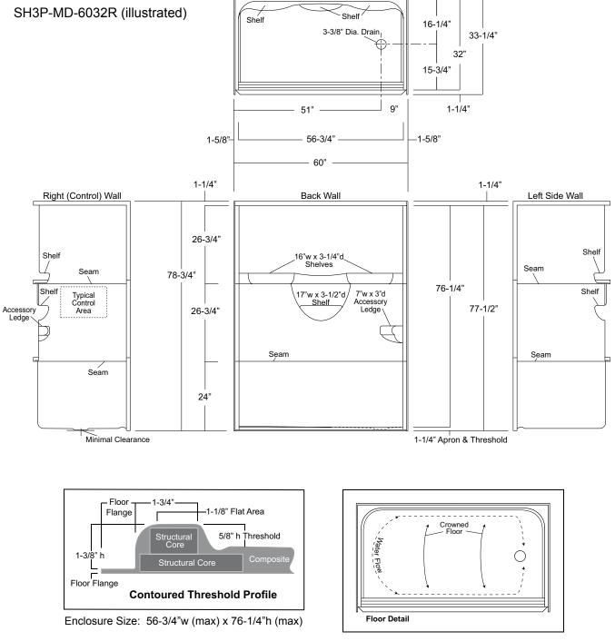
**NOTE:** Due to narrow threshold size and ramped configuration, care must be used in selecting an enclosure.
