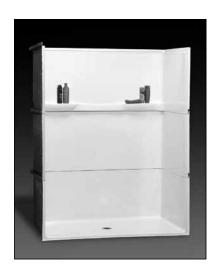
**Specification** – Oasis 3-piece FRP gelcoat shower compartment SH3P-6334, having a 60 x 30-inch minimum clear interior dimension and 7/16-inch high maximum finished threshold with floor attachment flange on lower threshold. An ActivLife factory-equipped package shall include 2-wall horizontal and single-wall vertical bar and seat reinforcement.
