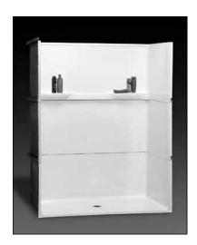
**Specification** – Oasis 3-piece FRP gelcoat shower compartment SH3P-6334, having a 60 x 30-inch minimum clear interior dimension and 7/16-inch high maximum finished threshold with floor attachment flange on lower threshold. An ActivLife factory-equipped package shall include 2-wall horizontal bar reinforcement and seat reinforcement.
