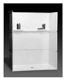
**Specification** – Oasis 3-piece FRP gelcoat shower compartment SH3P-6334, having a 60 x 30-inch minimum clear interior dimension and 7/16-inch high maximum finished threshold with floor attachment flange on lower threshold. An ActivLife factory-equipped package, exceeding Fair Housing requirements, shall include 3-wall horizontal bar reinforcement and 2-wall seat reinforcement.
