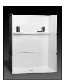
**Specification** – Oasis 3-piece FRP gelcoat shower compartment SH3P-6334, having a 60 x 30-inch minimum clear interior dimension and 7/16-inch high maximum finished threshold with floor attachment flange on lower threshold. ActivLife package includes factory applied, 3-wall, mid-level wrap reinforcement, exceeding (HUD/FHA) 'Fair Housing' requirements.
