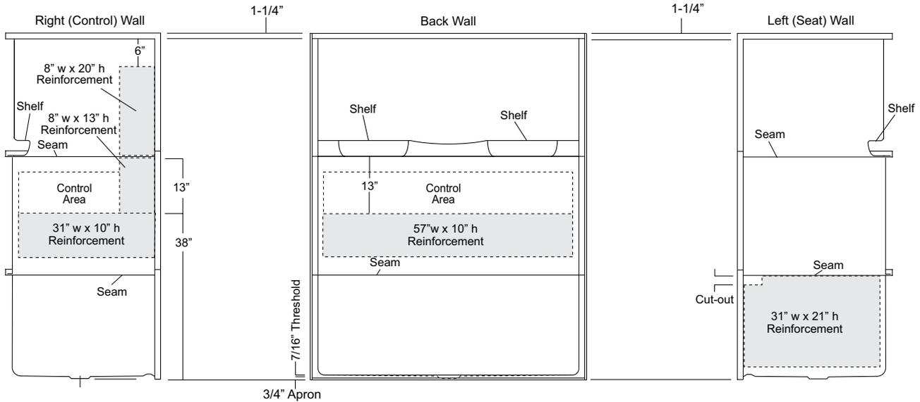
Package Order No.: TLRF-DS (3-wall bar & 2-wall seat reinforcement)
