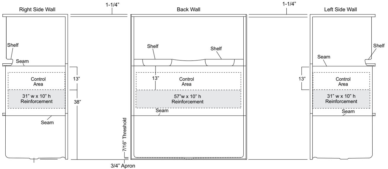
**Package Order No.: TLRF-RS or LS (2-wall bar & RH or LH seat reinforcement)**
