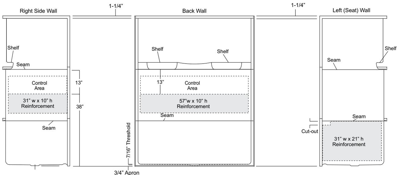
Package Order No.: TLVRF-RS or LS (2-wall bar & RH or LH seat reinforcement)
