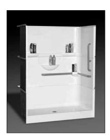
**Specification** – Oasis 3-piece FRP gelcoat shower compartment SH3P-6032 center drain shower with L or R control wall, offered in a standard 4-inch or 6-inch (ABF) dam configuration. ActivLife package includes a single horizontal bar on the back wall and control wall, and a vertical bar on the control wall.
