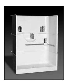
**Specification** – Oasis 3-piece FRP gelcoat shower compartment SH3P-6032 center drain shower with L or R control wall, offered in a standard 4-inch or 6-inch (ABF) dam configuration. ActivLife package includes a horizontal bar across the back wall and across the control wall.
