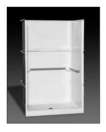
**Specification** – Oasis 3-piece FRP gelcoat shower compartment SH3P-4832, offered in a standard 4-inch or 6-inch (ABF) dam configuration. ActivLife package includes a horizontal bar across the back wall and across the control wall.
