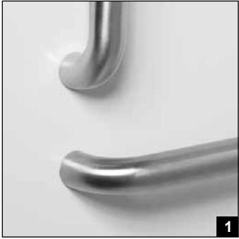
Photo 1: Grab Bars: Factory-installed 1.50-inch diameter, concealed attachment, 18 gauge, #304 brushed stainless steel grab bars. Concealed attachment design provides tamper-resistance and minimizes debris collection areas at contact points, compared to common exposed flange bar designs, without compromising bar attachment integrity. (Reinforced areas include a structural core material encapsulated in FRP composite.) Photo 2: Grab Bars: Factory-installed 1.25-inch dia. powder coated (in finishes listed above), concealed attachment, 18 gauge, #304 stainless steel grab bars. Concealed attachment design provides tamper-resistance and minimizes debris collection areas at contact points, compared to common exposed flange bar designs, without compromising bar attachment integrity. (Reinforced areas include a structural core material encapsulated in FRP composite.)
