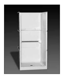
**Specification** – Oasis 3-piece FRP gelcoat shower compartment SH3P-3636, offered in a standard 4-inch or 6-inch (ABF) dam configuration. ActivLife package includes a single horizontal bar across the back wall.
