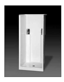
**Specification** – Oasis one-piece FRP gelcoat shower compartment SH-3232, offered in a standard 4-inch or 6-inch (ABF) dam configuration. ActivLife package includes factory applied, 3-wall, full-wrap reinforcement, exceeding (HUD/FHA) 'Fair Housing' requirements.
