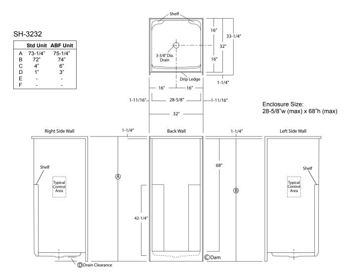
NOTE: This model is non-conforming in size and has less than a 900 square-inch interior area.
