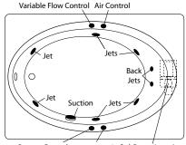
System Control Air Control Std. Pump Location
