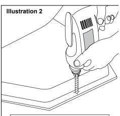
Drill base flange at various joist locations and lag to floor structure.
