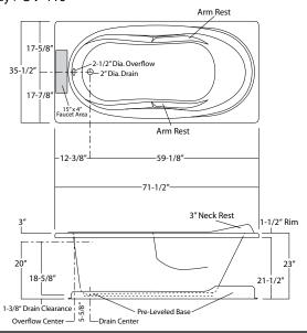
NOTE: A pump access MUST BE PROVIDED for all whirlpool equipped units. Additional access may be required to comply with local codes.
