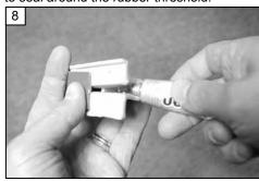
Remove the adhesive backing and apply E-6000 around the perimeter of the end cap.
