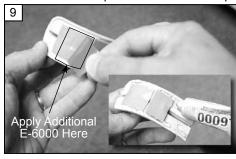
NOTE: In some installations, an exact fit of the end cap to the unit corner is not attainable and additional E-6000 adhesive should be applied as noted in images 9 & 10.
