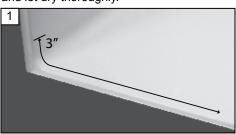
With a pencil, mark the shower floor inward from the front edge ½-inch. Repeat in the middle and on the opposite end. Using a straight edge draw a line between the pencil marks. This is your front edge alignment line. NOTE: If installing on an SHFW model, skip this step and proceed to step 3.
