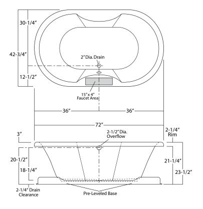
Sump Dimen: 50" long x 28" wide x 20-5/8" deep Sump Capacity: 88 gal. (unoccupied - to overflow)
