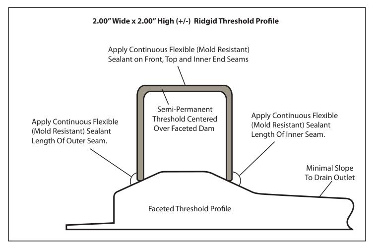
Note: Semi-permanent threshold offered, as an option, on 1.25" faceted threshold models, and is designed for independent field application and removal by others.
