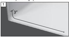
With a pencil, mark the shower floor inward from the front edge ½-inch. Repeat in the middle and on the opposite end. With a straight edge draw a line between the pencil marks. This is your front edge alignment line.
