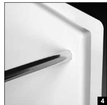
Photo 1: Grab Bars: Factory-installed 1.50-inch diameter, concealed attachment, 18 gauge, #304 brushed stainless steel grab bars. Concealed attachment design provides tamper-resistance and minimizes debris collection areas at contact points, compared to common exposed flange bar designs, without compromising bar attachment integrity. (Reinforced areas include a structural core material encapsulated in FRP composite.)
